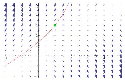
we see that a solution to the initial value problem y' = y - x, y(1) = 3 passes through the point (1.3) and follows the direction of the arrows.
