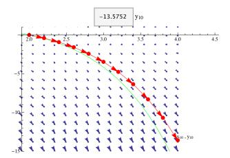
In the above picture, we show the approximate solution in red alongside the real solution to the Initial value problem in green. In general a smaller step size should give a more accurate approximation.
